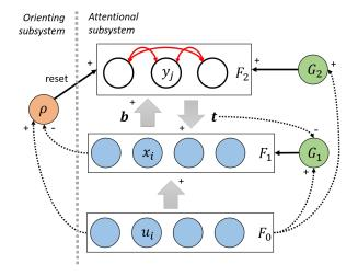
Gain units  $G_l$  serve to switch operational phases in the  $F_l$  layer
