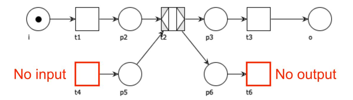
Not a workflow net (not all nodes are on a path from i to o)
