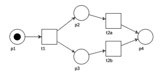
(when a token is in the final place the case should end) can arise in workflow nets
