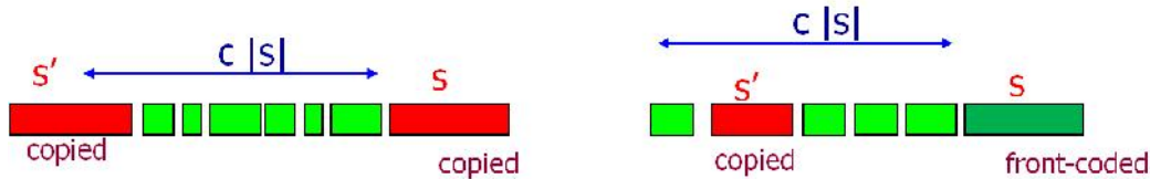
FIGURE 7.4: The two cases occurring in LPFC. Red rectangles are copied strings, green rectangles are front-coded strings.
