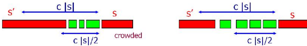
FIGURE 7.5: The two cases occurring in LPFC. The green rectangles denote the front-coded strings, and thus their FC-characters, the red rectangles denote the two consecutive copied strings.
