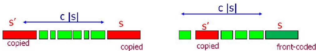
FIGURE 7.4: The two cases occurring in LPFC. Red rectangles are copied strings, green rectangles are front-coded strings.
