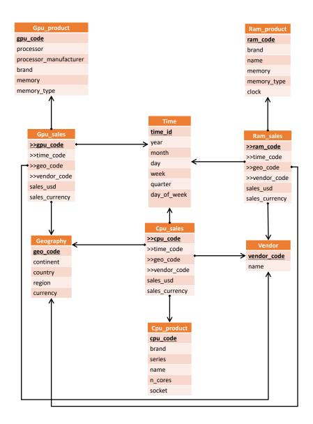
Figure 1: Datawarehouse schema of reference.
