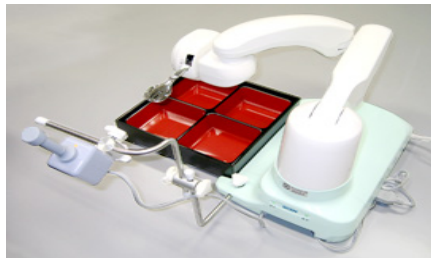
Figure: meal support robot [4]
